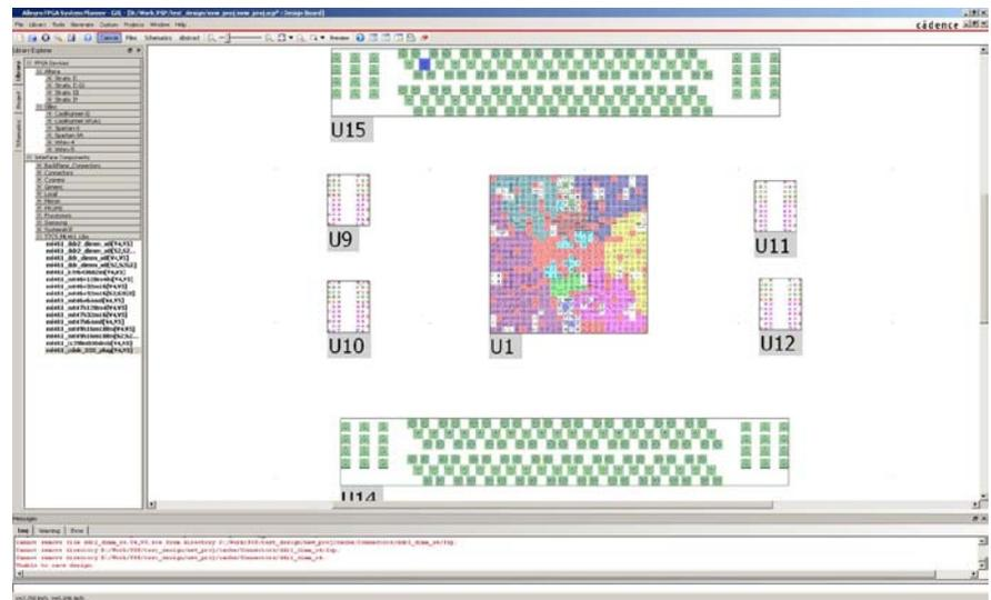
Figure 2: Placement/Floorplan view of the OrCAD FPGA System Planner provides users relative placement of critical components for optimum pin assignment synthesis
