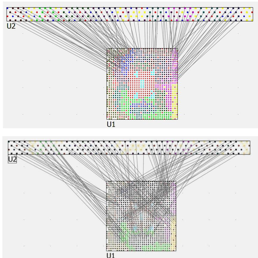
Figure 4: OrCAD FPGA System Planner optimization
