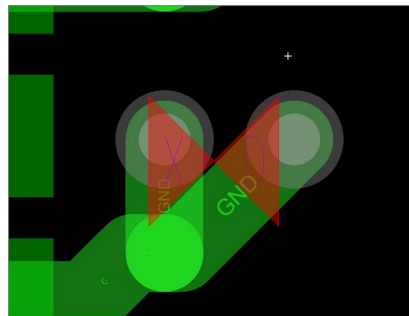
Figure 2. Acid trap violation
